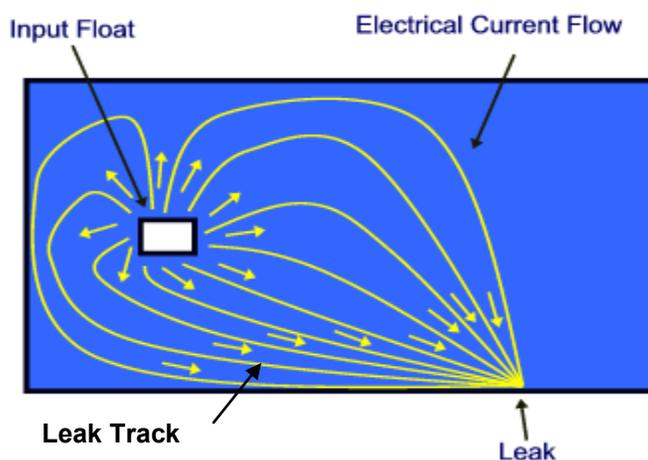
The sophisticated LeakTrac 2400 detects these “Leak Tracks”, by measuring the differential voltage potential at different points in the pool, and translates this information into audible clicking sounds that increase in frequency as the voltage differential increases.
