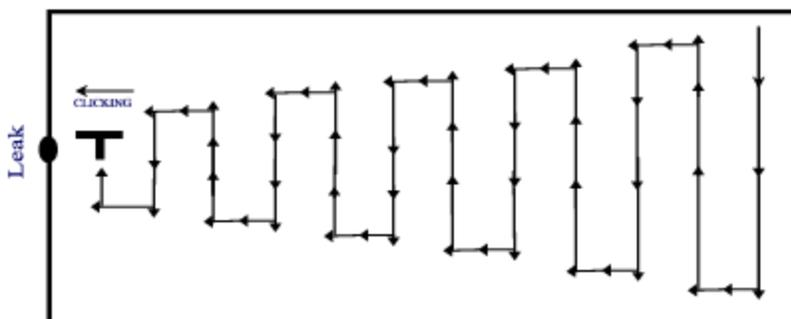
Most leaks are discovered as you are moving the probe in the direction producing a whine then all of a sudden the signal stops. This indicates that the probe has passed over the leak and is now pointing away. Turn the probe around and carefully examine the area just passed.
