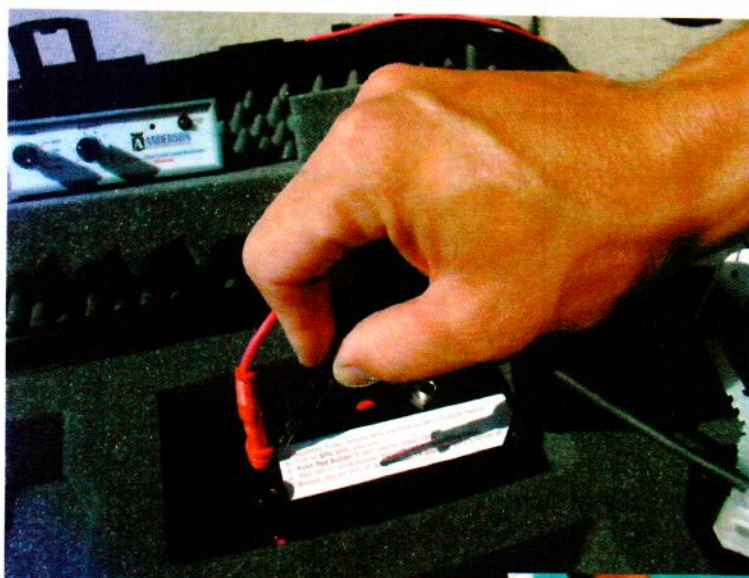
Above: 'Ground' and 'Input' cables are plugged into a battery-powered booster to produce detectable electrical current flow.
