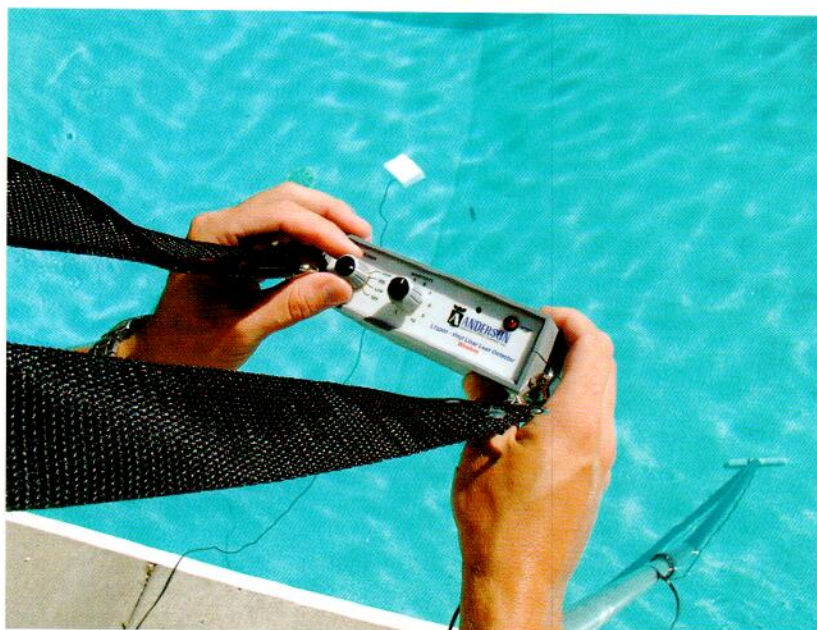
Above: A signal processing unit produces an audible clicking sound when the probe is pointed in the direction of electrical flow.
