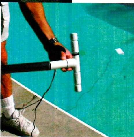
Above: 'Ground' and 'Input' cables are plugged into a battery-powered booster to produce detectable electrical current flow.
