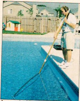
A new vinyl-liner leak locator.
