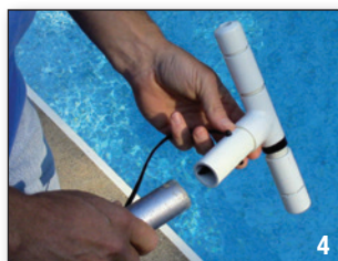
4 The "Probe" attaches to the end of a standard telescopic pole. It is then plugged into the back of the SPU.
