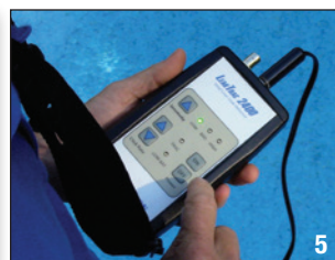
5 The simple to operate SPU produces an audible clicking tone when the probe is pointed in the direction of the electrical flow.
