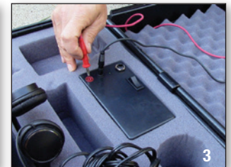
3 Plug "Ground" and "Input" cables into the battery powered "Booster" that produces the detectable electrical current flow.
