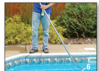
6 As the "Probe" is brought closer to a leak the clicking increases in frequency allowing leaks to be pinpointed in minutes.
