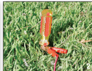
2 Attach the "Ground Cable" to a grounded object outside the pool. A ladder anchor, diving board anchor or ground stake will work.
