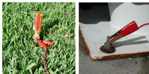
If the ground you choose is painted, you must scrape through the paint to assure an electrical connection is made with the ground clamp.
